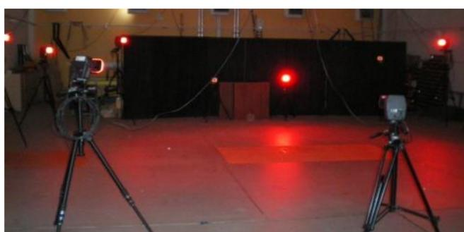
**Figure 2:** University of Sydney Laboratory set-up to collect gait data.
